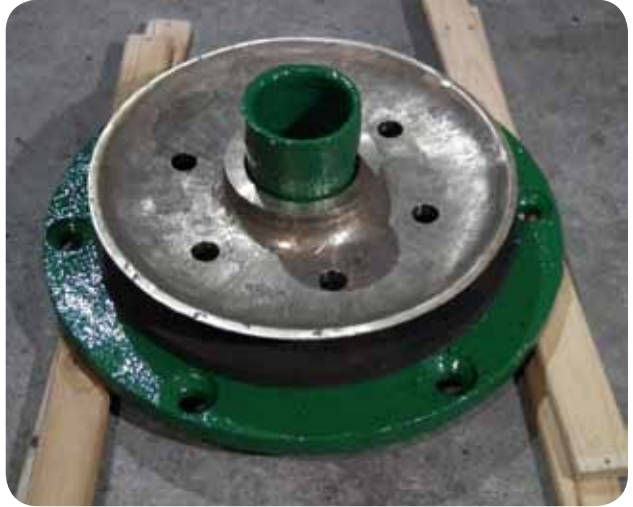
The rubber diaphragm and main casting.
