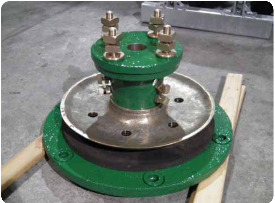
The fully assembled air pump valve.
